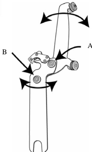
Loosen Allen Bolts A & B to adjust angle, then re-tighten Allen Bolts.
