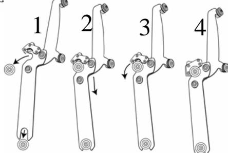
1. Place lower slot into lower bushing. 2. Rotate top slot into place. 3. & 4. Secure locking Mechanism.
