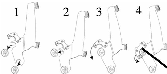
1. Place lower slot into lower bushing. 2. Rotate top slot into place. 3. & 4. Secure locking Mechanism.
