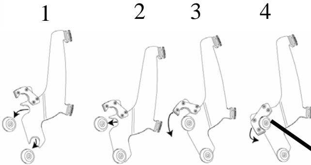
1. Place lower slot into lower bushing. 2. Rotate top slot into place. 3. & 4. Secure locking Mechanism.
