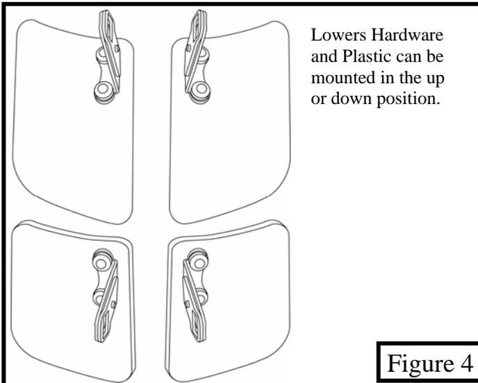
Lowers Hardware and Plastic can be mounted in the up or down position.
