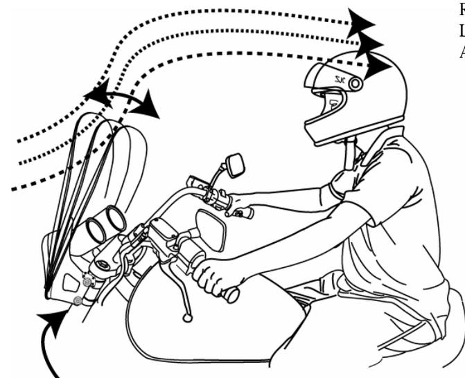
Loosen Allen Bolt to adjust angle, then re-tighten Allen Bolt.
