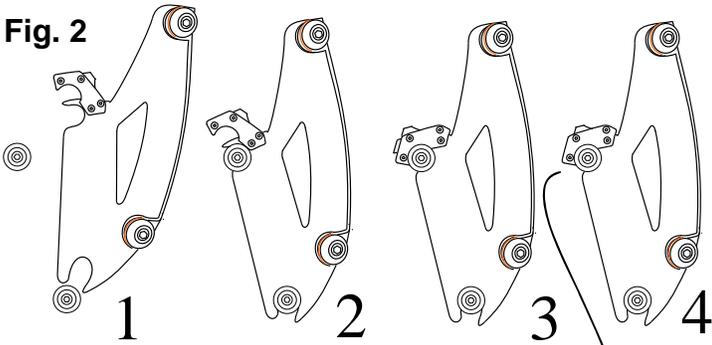
1. Place lower slot into lower bushing.
