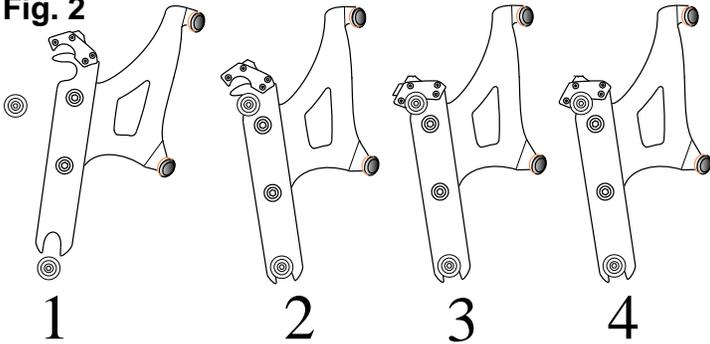
1. Place lower slot into lower bushing.
