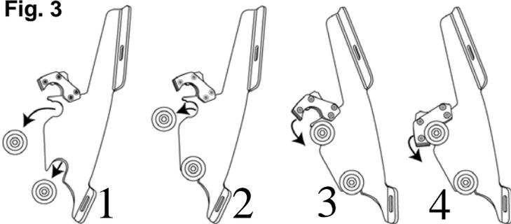
1. Place lower slot into lower bushing.
