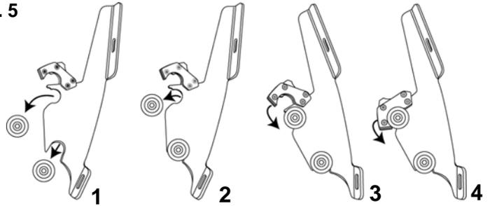
1. Place lower slot into lower bushing.
