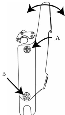
Loosen Allen Bolts A & B to adjust angle, then re-tighten Allen Bolts.
