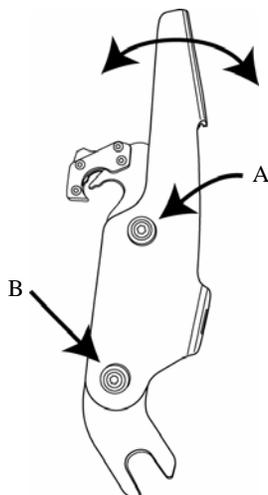
Loosen Allen Bolts A & B to adjust angle, then re-tighten Allen Bolts.
