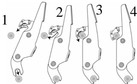
1. Place lower slot into lower bushing. 2. Rotate top slot into place. 3. & 4. Secure locking Mechanism.
