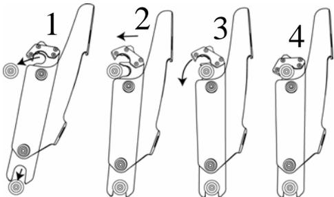
1. Place lower slot into lower bushing. 2. Rotate top slot into place. 3. & 4. Secure locking Mechanism.
