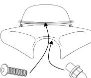
Remove the existing Acorn Nut Shoulder Spacers from the left and right holes. Withdraw the bolts and washers.
