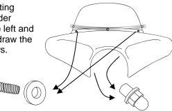
Align the Trim over the left and right holes and insert Button Head Screws.
