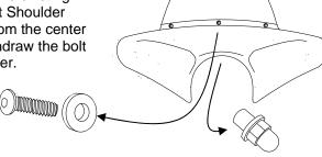
Align the Trim over the center hole and insert a Button Head Screw . Secure in place with an Acorn Nut Shoulder Spacer
