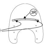
3. Line up the 3 hole front strap with the horizontal holes on the front of the windshield. Push a large socket spacer through the front strap, and into the hole in the windshield, at the location shown. Push a cap screw through each spacer and through the 3 hole rear strap. Slide a plastic spacer washer over the protruding threads and secure loosely with an acorn nut.
