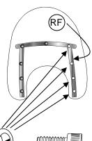
Make sure all of the straps are correctly lined up, then tighten down all of the bolts using a wrench (not supplied) and the 3/16" short arm allen wrench provided.
