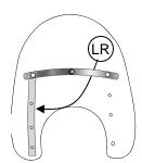
5. Line up the Left front strap with the left set of vertical holes on the front of the windshield. Push a large socket spacer through the front strap, and into the holes in the windshield, at the locations shown. Push a cap screw through each spacer and through the 3 hole rear strap. Slide a plastic spacer washer over the protruding threads and secure loosely with an acorn nut.
