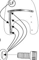
Line up the Right rear strap with the right set of vertical holes on the rear of the windshield. The step on the right rear strap sits over the 3 hole rear strap.
